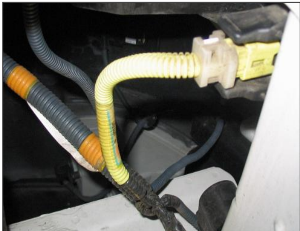
Example SRS Wiring (yellow)
